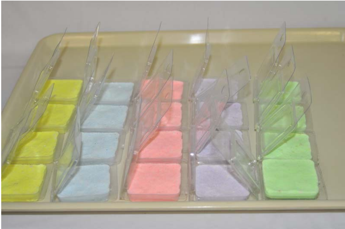
These are the plastic containers I used as moulds. They originally contained small screws. Other people go through supermarkets and see products, I see potential moulds ☺
